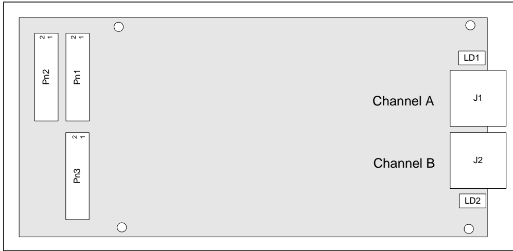
Figure 3 : Connector and LED Locations for the Copper FP PMC GE Adapter
