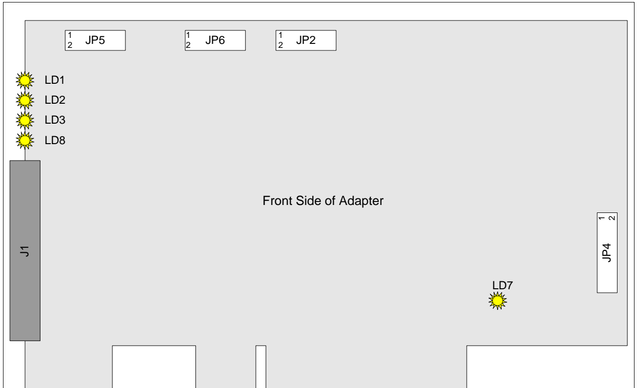
Figure 7 : Connector Locations on the HSS8 PCI and HSS4NG PCI Adapters (FP)
