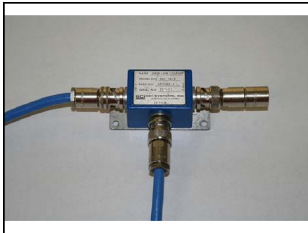
Figure 17 : Transformer Coupled, Terminated
