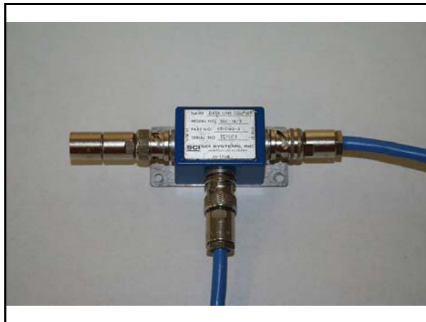
Figure 14 : Transformer Coupled, Terminated
